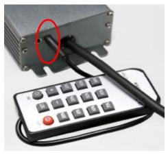
Firstly press to unlock, within 10s, press fuction key to adjust your required output current
