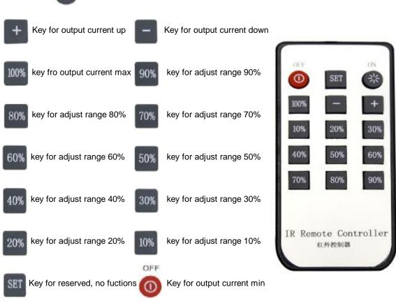
Warning: Please do not continuously press"+" to avoid the over power protection and unstable output.
